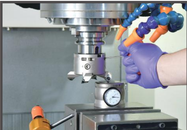
停機測量，占用主軸時間 Do measurement on cnc machine. Take time and idle the machine.
